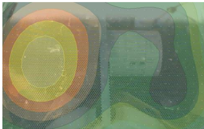
Figure 6. Acoustical holography image of engine compartment
